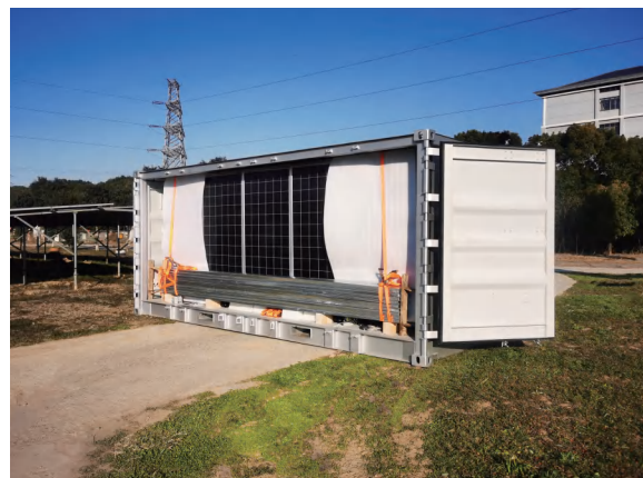
③ 开箱铺设 Open & Assembly
